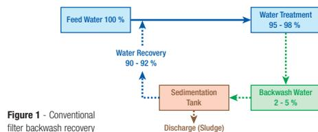
Figure 1 - Conventional filter backwash recovery
