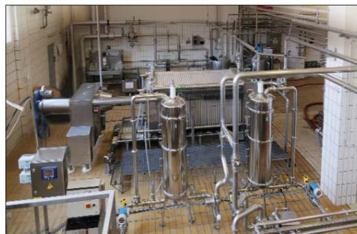
With the flat filter sheets having 170 m<sup>2</sup> (1829 ft<sup>2</sup>) filtration area, 10,250 hl (270,776 USg) of beer could be filtered, equivalent to 60.3 hl/m<sup>2</sup> (148.0 USg / ft<sup>2</sup>). With the 12 SUPRAPak modules in two compact closed system housings, a total volume of 16,240 hl (429,015 USg) (related to 10 filtrations/ sterilizations, which is recommended by Pall) could be filtered, equivalent to 1,353 hl/module (35,742 USg/module).
